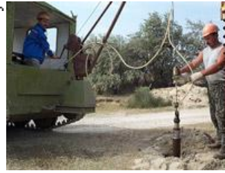
Borehole air-operated wave transducer «Puls 6C» Placing of airgun into the well hole
